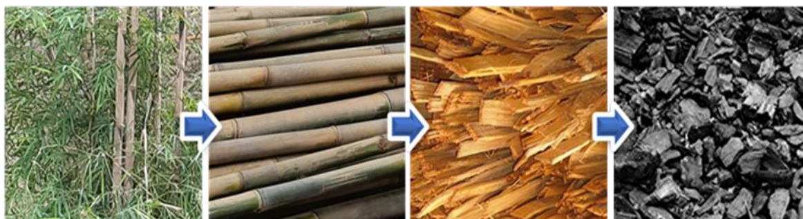
Figure 1. The steps in producing bamboo charcoal. Left to right is bamboo tree, pieces of bamboo internodes, chopped and dried bamboo, and bamboo charcoal
